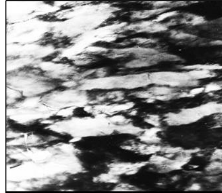
a b Fig. 4 Substructure of steel before (a) and after (b) IB; × 15000.
