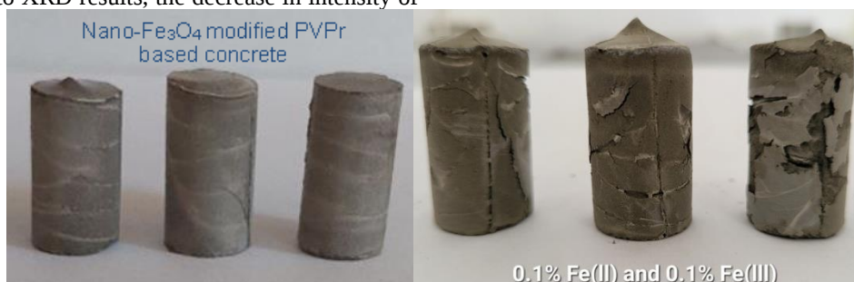
Fig 6. Concrete samples filled with magnetite nanoparticles PVPr and \text{Fe}^{2+}/\text{Fe}^{3+} salts after 28 days of curing.
