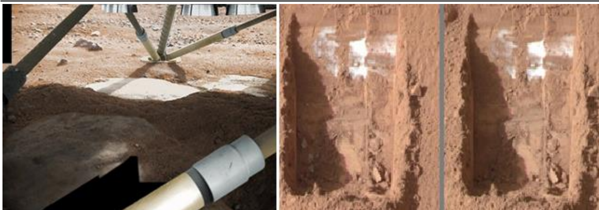
Fig. 1. Left – the engines of the Phoenix lander blew away the upper layer of dust and exposed the frozen water ice. On the right – ice under the "shovel" of the "Phoenix" module ( http://photojournal.jpl.nasa.gov/ ).
